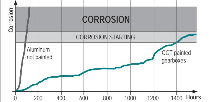
This graph is an indication, since some chemical components may be more aggressive than the salt spray test. Tests are suggested on special cases (in case use type "N series", full stainless steel gearboxes).
